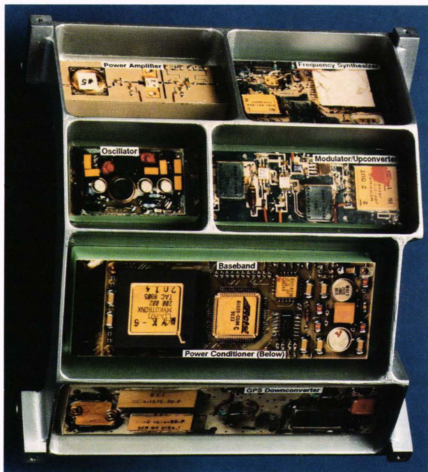
Figure 10. Global Positioning System Translator and Telemetry (GTT) Transmitter electronic assembly.
