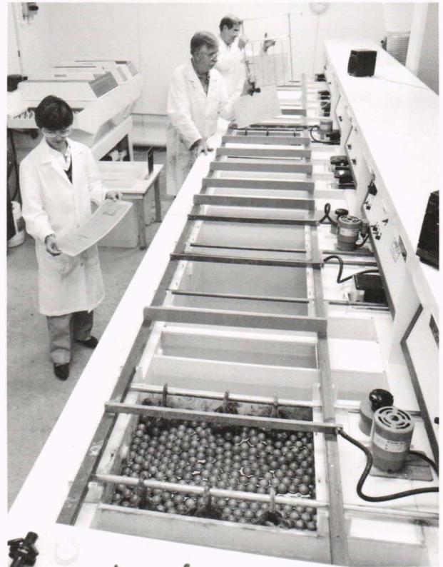
Figure 4. Process tanks used to plate copper, tin, lead, nickel, and gold on printed wiring board substrates.
