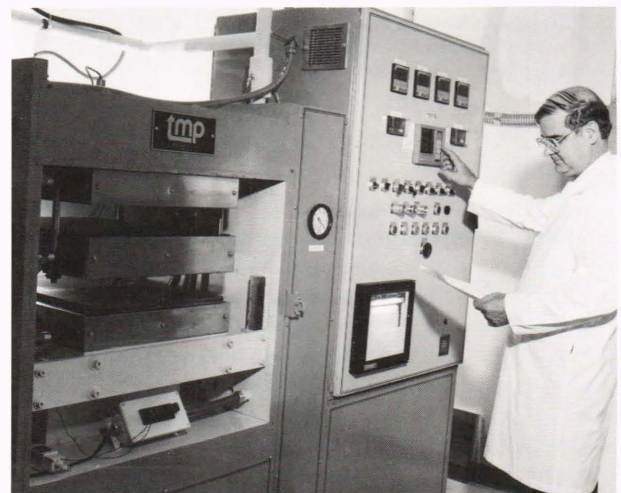
Figure 5. A computer-controlled 100-ton hydraulic press with a vacuum chamber for laminating multilayer boards.
