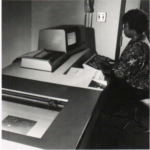
Figure 10. A technician programs a computer to test a circuit board for undesired open and short circuits by using test files generated by computer-aided design.
