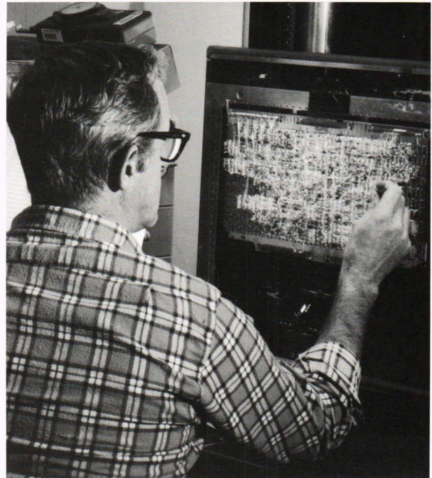
Figure 6. A numerically controlled wire wrap tool positions terminals and provides properly cut and stripped wire by using instructions from computer-aided design/computer-aided engineering tools.
