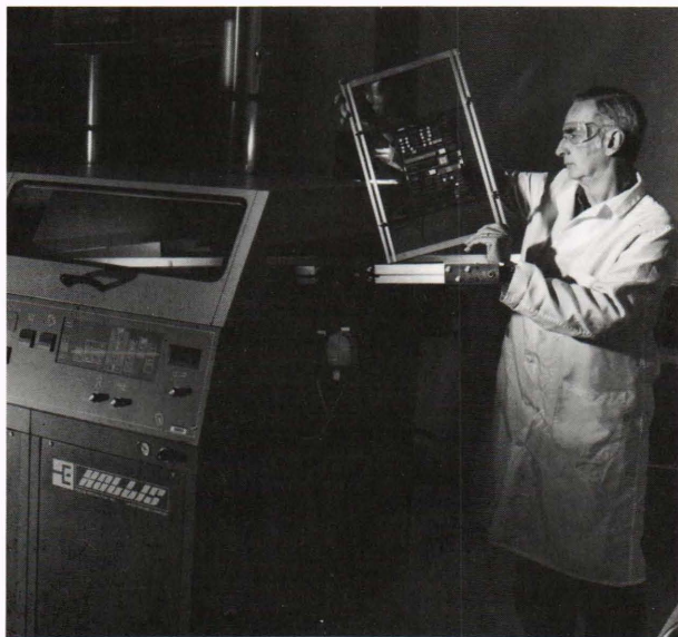
Figure 11. A dual-wave soldering machine attaches bottom-surface-mounted and all through-hole components in one pass.
