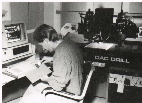
Figure 3. An operator of a computer numerically controlled drill/router examines the drilling instruction file received from a computer-aided design tool.
