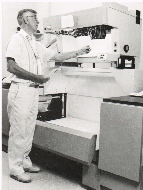
Figure 5. Aperture card production. Drawings are photographed and aperture cards are filed for future reference.
