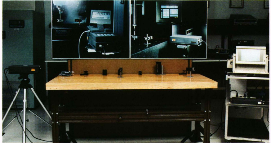
Figure 1. The Renishaw laser interferometer test set-up measures machine tool alignment and calibration.
