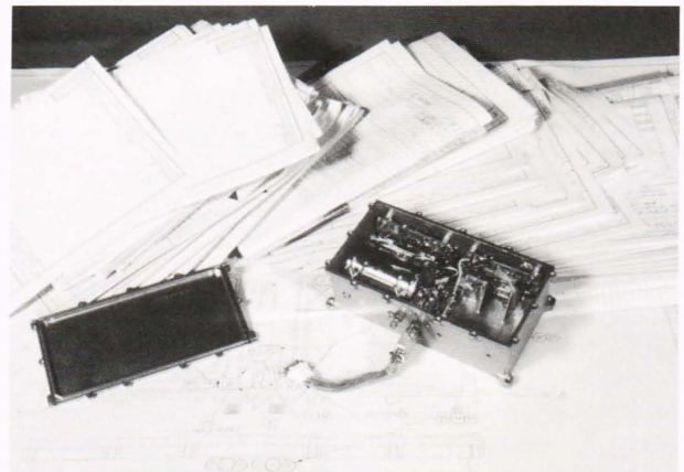
Figure 8. Example of the documentation package necessary to create flight electronics hardware such as the 5-MHz ultrastable oscillator shown here.
