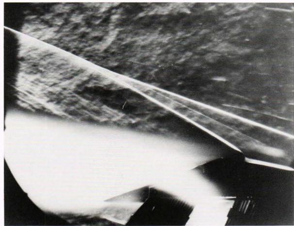
**Figure 8.** Supersonic combustion at the rear of an external-burning ramjet model is shown in this schlieren photograph taken in a Mach 5 flow. The double wedge model is upside-down, with its knee pointing upward, and the air flows from right to left. The first shock wave is produced by the model's leading edge (out of view). The second shock is caused by the injection of fuel. The bright region is due to the emission of light from the flame.
