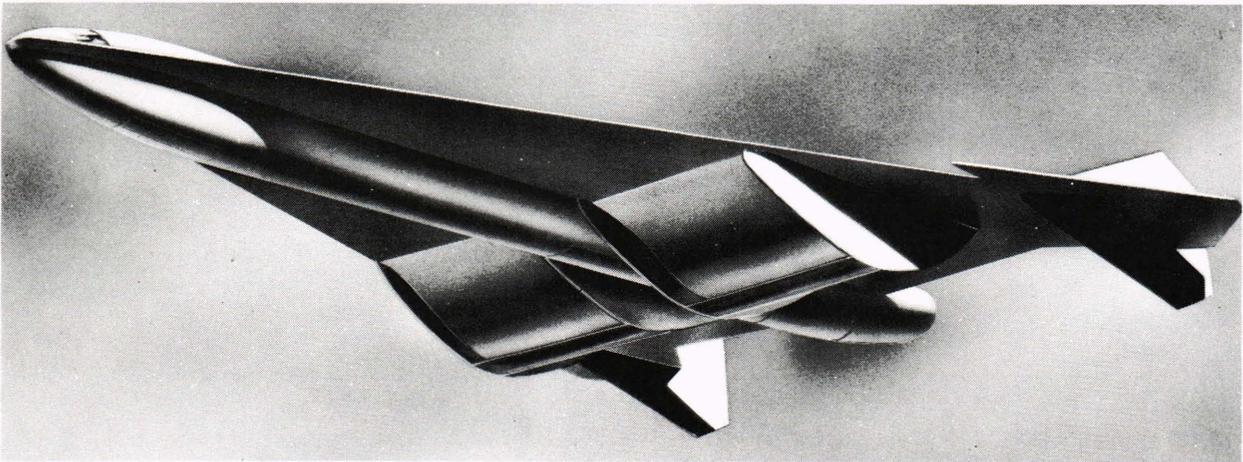
**Figure 15.** The principal configuration of the APL hypersonic transport was a 175-foot-long delta-winged aircraft with a wing span of 102 feet. It used turbojet engines to accelerate to Mach 3.6 and external expansion ramjets for propulsion at higher speeds, up to a cruise Mach number of 7. In the lower-speed range, the inlet ramps of the ramjet engine retracted to provide an opening for airflow to the turbojets.
