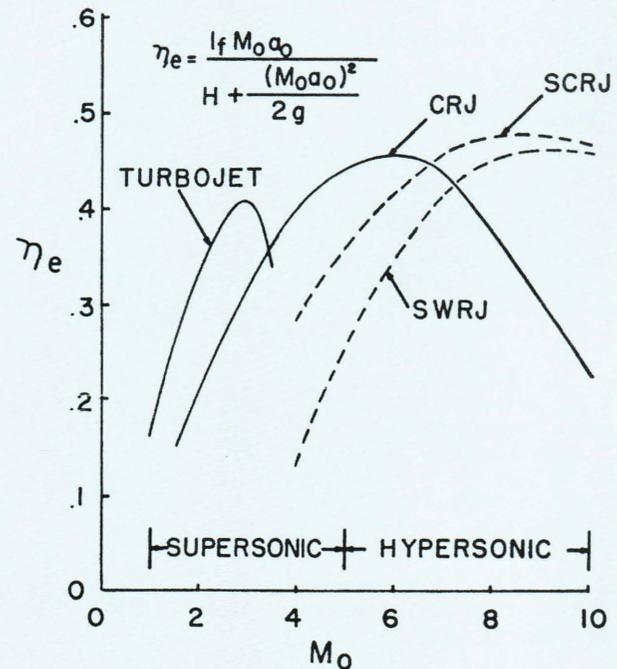
Figure III. Efficiencies for airbreathing engines. CRJ = conventional ramjet, SCRJ = supersonic-combustion ramjet, SWRJ = standing-wave ramjet.
