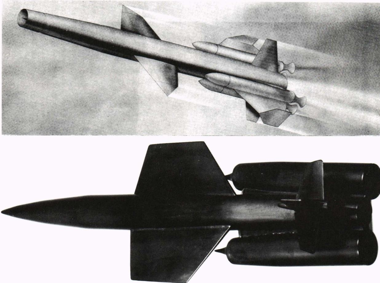
**Figure 3.** (Top) This 1951 drawing shows the early design concept of Triton, a very large missile intended for launching at sea. (Bottom) A wind-tunnel model of a later version, with its two ramjet engines mounted in the high-pressure region under the wings. The Triton program was canceled in 1958.
