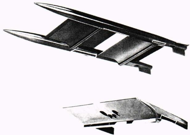
**Figure 16.** The hypersonic transport configuration shown in the upper part of this figure employed a highly staggered biplane design to control the movement of the center of pressure during large changes in speed, and to allow a high degree of engine/wing integration. The configuration in the lower part of the figure is a flying-wing (or a flying-engine), with passengers seated within the wing itself. Pectoral flaps extended from the sides for takeoff and landing.
