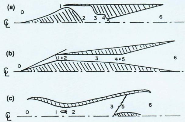
Figure II. Hypersonic ramjet forms. (a) Conventional ramjet. (b) Supersonic-combustion ramjet. (c) Standing-wave ramjet.
