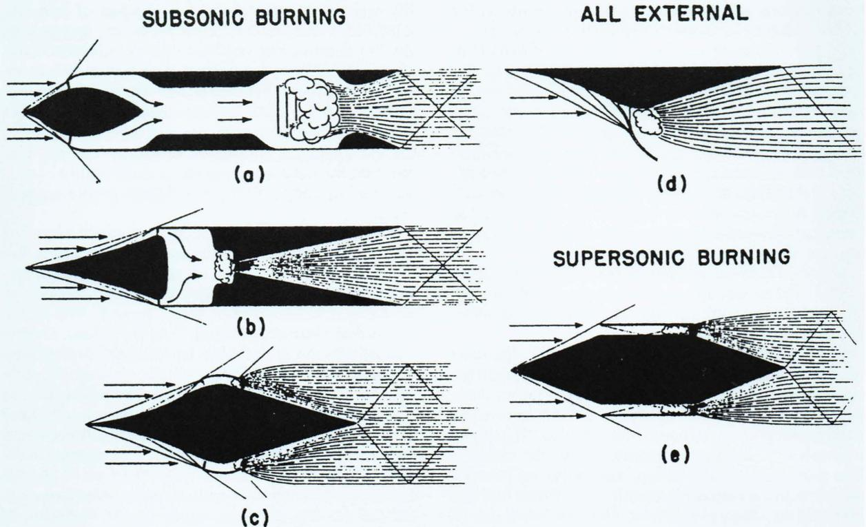
**Figure I.** Possible paths of evolution for the hypersonic ramjet. (a) Conventional ramjet engine. (b) High-speed subsonic-combustion ramjet. (c) External expansion ramjet. (d) Pure external ramjet. (e) Supersonic-combustion ramjet.
