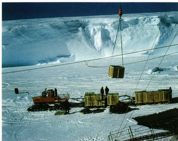
Figure 7. Cargo operations at Mobster Creek, showing the sledges being loaded with cargo from the ship.
