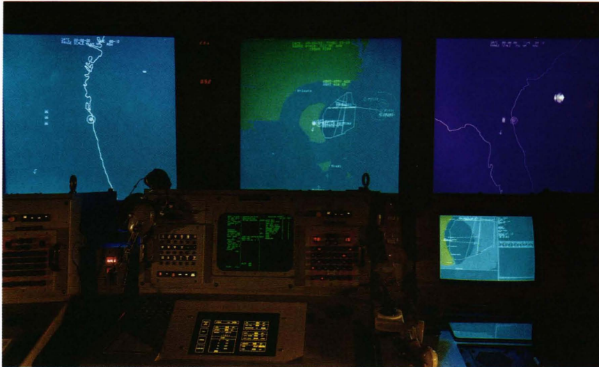
Figure 6. Experimental displays of the Command Support at Sea Experiments (CS@SE). This rapid prototyping effort employs commercial equipment and computer programming facilities to implement necessary or highly desirable features.
