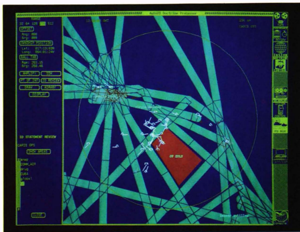
Figure 8. Operator display of the Automatic Identification System.
