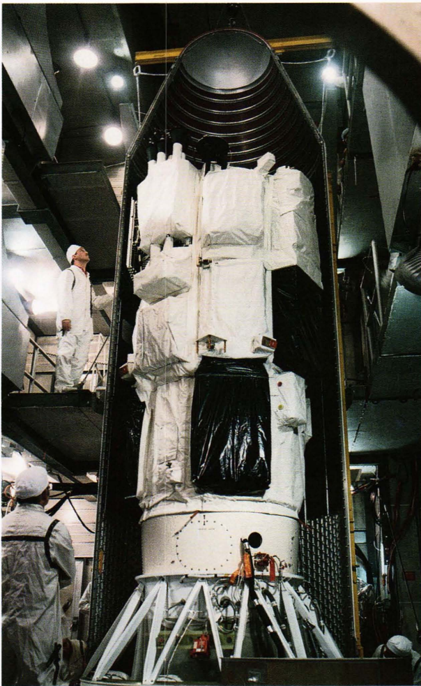
Figure 7. The heat shield being installed on the integrated Delta 181 Sensor Module. Thermal blankets cover the spacecraft.
