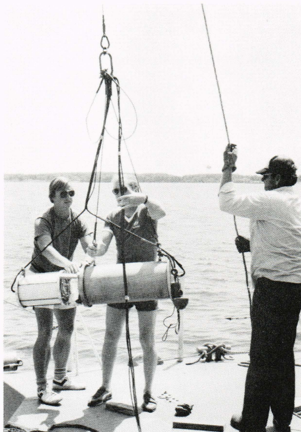
Figure 7. Aboard R/V Ridgely Warfield during an oxygen depletion study, crewmen prepare a waterproof bio-optical video system for lowering over the side. The chamber on the left houses a parallel light source that projects shadowgraph images of small sea-life passing through the gap. The video camera is housed in the large chamber.
