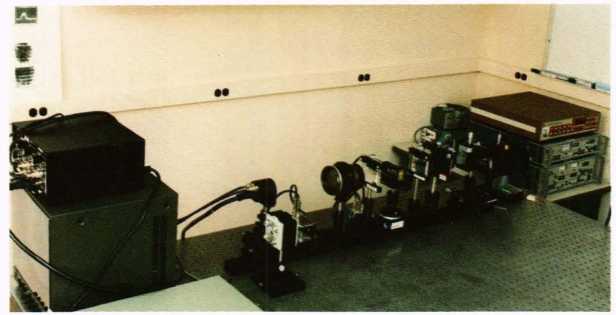
Figure 12—Photograph of the one-dimensional, acousto-optic, Bragg-cell spectrum analyzer.
