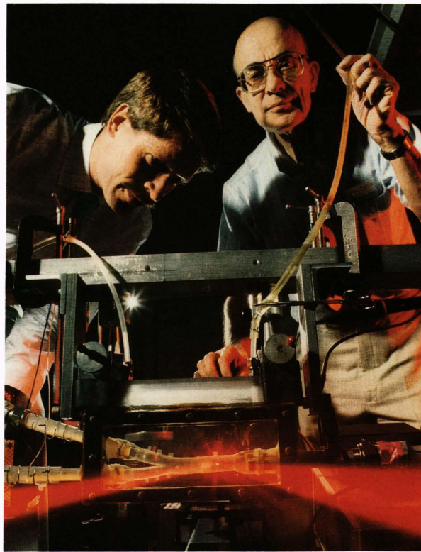
Figure 2 —Donald Duncan (left) and F. Fausten Mark making laser Doppler velocimeter measurements of simulated blood flow. The crossed laser beams of the velocimeter are seen emerging from the model of a segment of artery. Further information is given in the article by Duncan.
