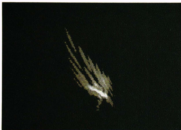
Figure 11 —Blurred image of the point source caused by substitution of a common lens for the custom-made lens now in the vector magnetograph.
