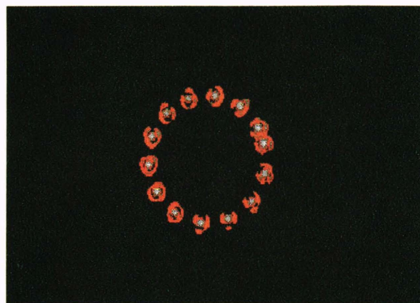
Figure 12 —Effect of prism rotation on the image of a point source of light. Note the astigmatism, shown by the nonuniformity of the diffraction ring.
