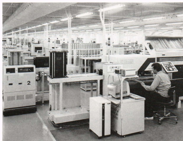
Figure 6 —Automated component insertion at Fujitsu. Robotic component insertion into printed circuit boards is accomplished with a minimum of human intervention.
