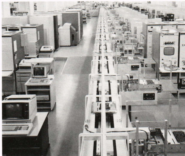
Figure 5 —Automated unit testing at Fujitsu, with each stage of the manufacturing process using electronic controls and sensors to assure quality.
