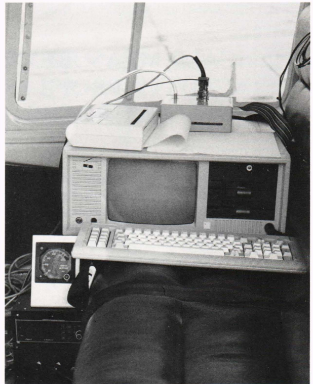
Figure 2 —The data acquisition computer and sensor electronics strapped to the rear seat of the helicopter.
