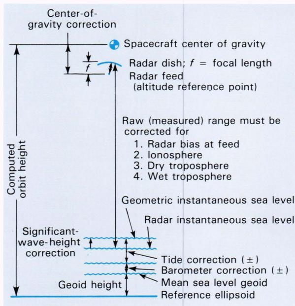
Figure 1—Altimeter data reduction.
