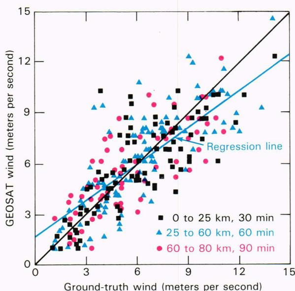
Figure 2—A comparison between GEOSAT and ground-truth station winds at 10 meters.
