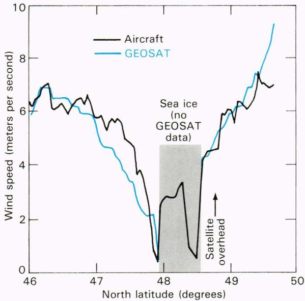
Figure 7—A comparison between GEOSAT and Adaptive Wind/Wave Radar System winds for April 24, 1985.
