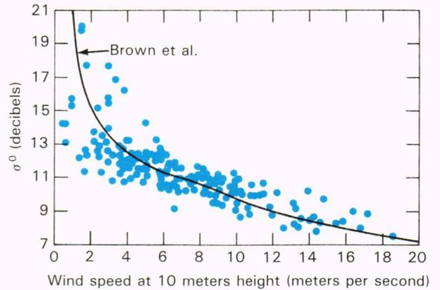
Figure 3—GEOS-3  $\sigma^0$  versus ground-truth wind speed at 10 meters. The solid curve is the Brown et al. wind model.<sup>1</sup>
