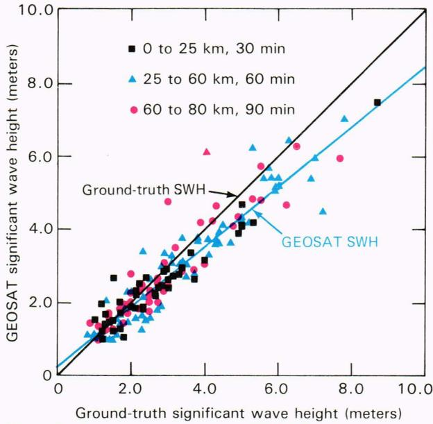
Figure 6—A comparison between GEOSAT and ground-truth significant wave height.
