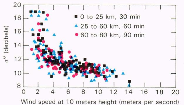
Figure 4—GEOSAT  $\sigma^0$  versus ground-truth wind speed at 10 meters.
