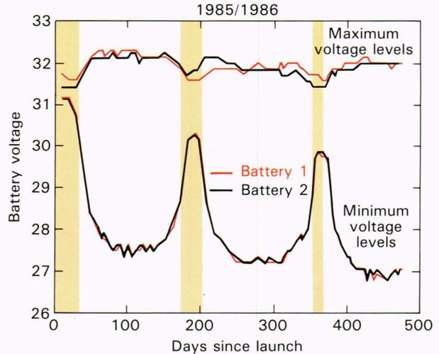
**Figure 8**—Battery voltage performance. The shaded area shows the sunlit orbit, and the unshaded area shows the partially eclipsed orbit.
