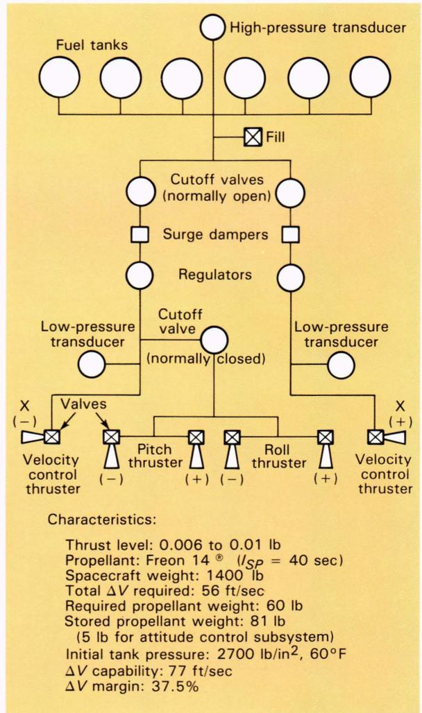
Figure 5—Schematic diagram of the velocity control system.
