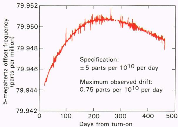
Figure 7—The drift of the 5-megahertz oscillator frequency of the Doppler beacon.
