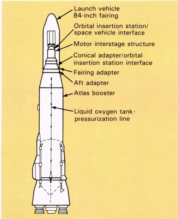
Figure 3—Launch vehicle configuration.
