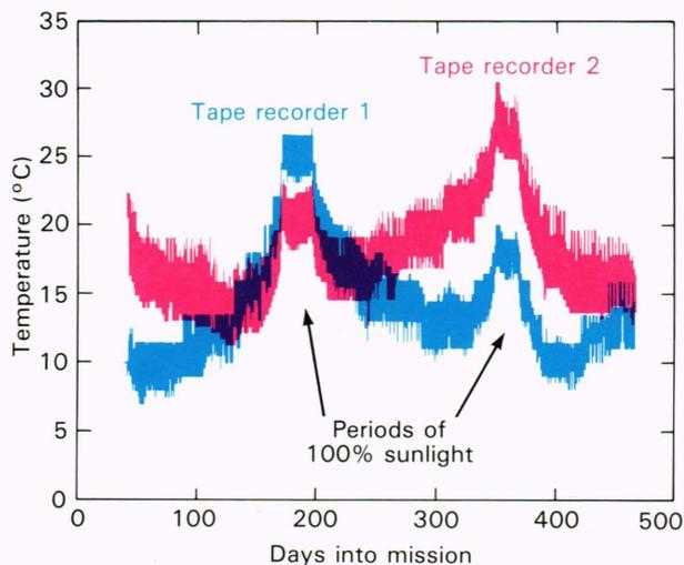
Figure 6—External temperatures of the tape recorders.
