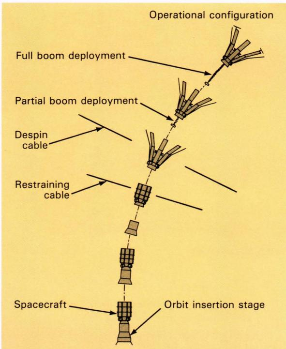
Figure 4—Orbit insertion phase.
