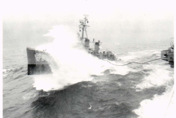
Figure 1—Pitching motion, keel slamming, and sea spray while refueling in moderate to heaving seas, April 1962.
