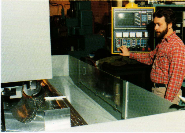
Figure 4 —An experimental machinist using the custom cutter in the Cincinnati 10VC numerical control vertical machining center to machine the cornu-bend mold half.
