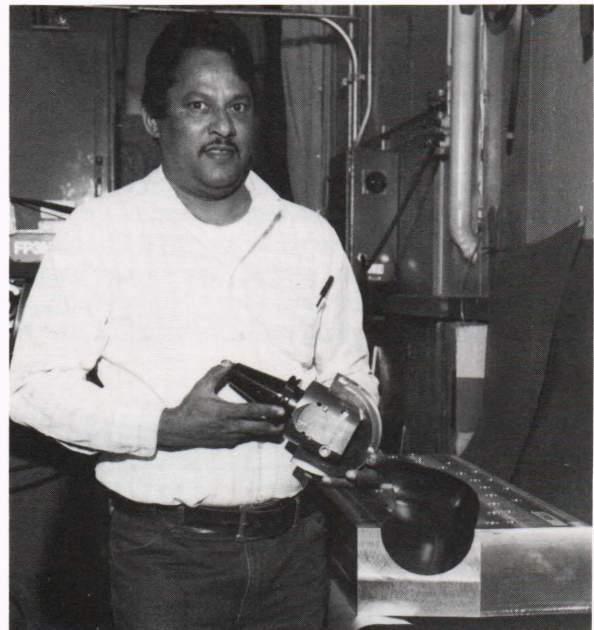
Figure 3—A tool and cutter grinder with a custom two-flute cutter he fabricated in order to machine the mold half shown on his left.
