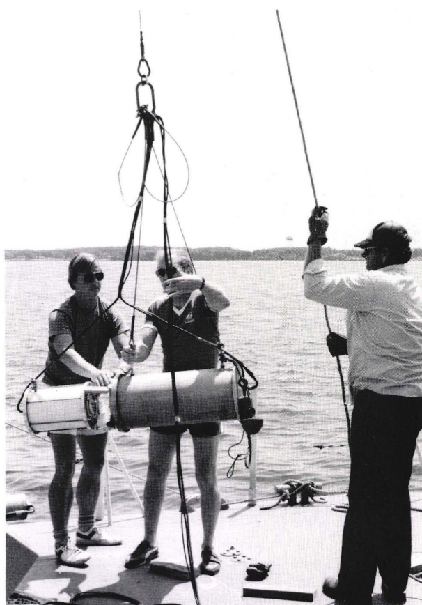
Aboard R/V Ridgely Warfield during an oxygen depletion study, crewmen prepare a waterproof bio-optical video system for lowering over the side. Joe Hopkins of APL, center, developed the system. The chamber at left houses a parallel light source that projects shadowgraph images of small sea life passing through the gap. The video camera is housed in the large chamber. Crewmen, left to right, are Randy Loftus and Doug Hallock.
