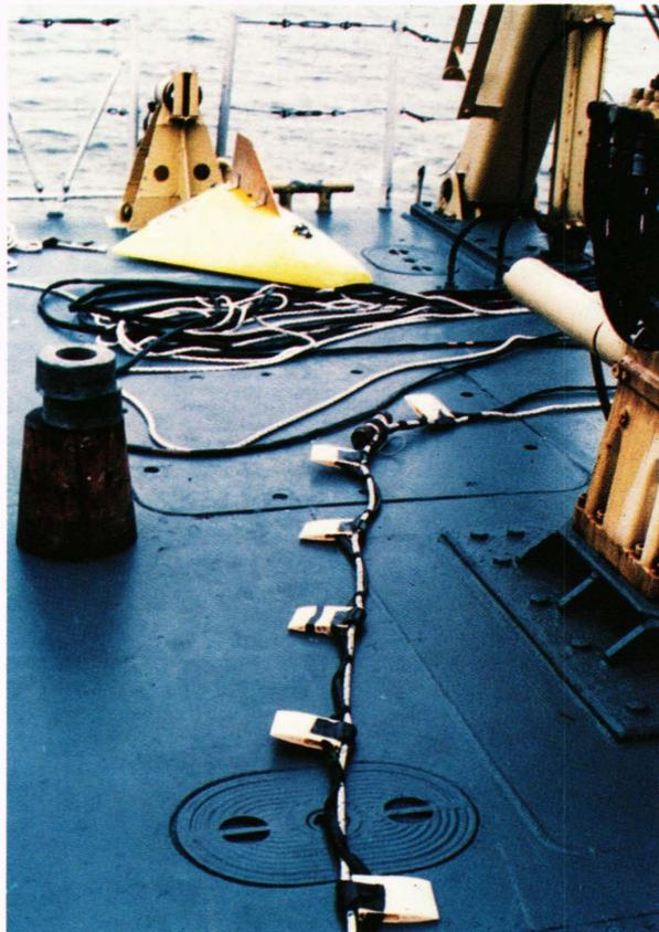
**Figure 10**—Thermistor-chain system, which measures the temperature fluctuations associated with vertical displacements of the water column. The observed temperature fluctuations are indicative of internal-wave and turbulent mixing activity.
