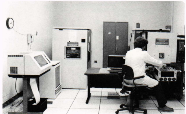
Figure 7 —The digital large-scale-integration test station. Incoming parts such as digital integrated circuits are tested here before being placed in stock to be used in space hardware.
