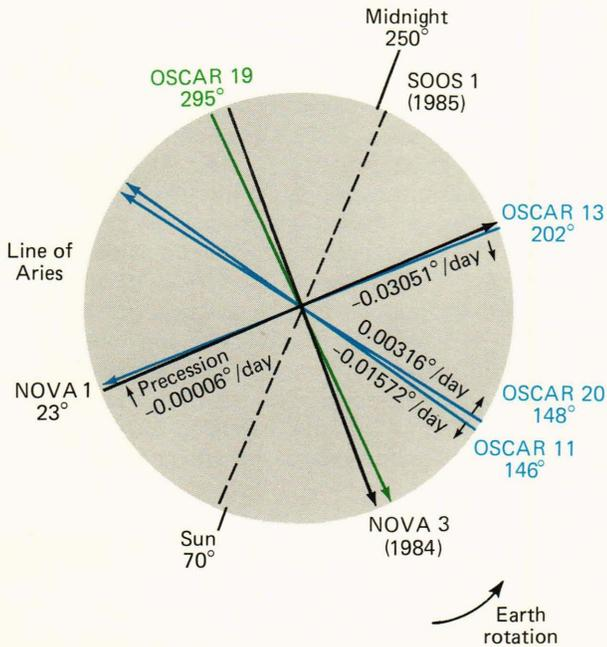
**Figure 3**—View of the operational TRANSIT constellation in October 1984 as seen from a position above the north pole. Because of recent battery cell failures, OSCAR 19 provides service only in full and near-full sun. Planned launch orbits are shown with dotted lines.
