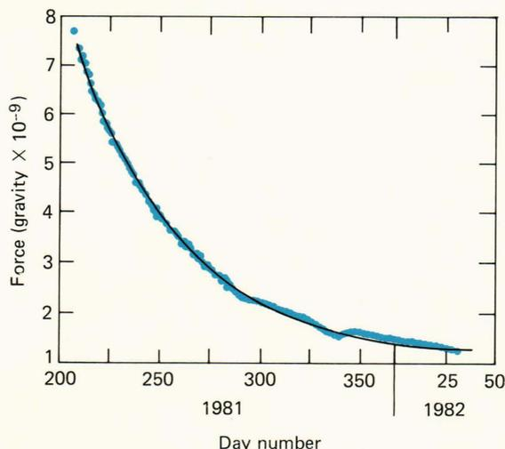
**Figure 5**—Approximately 200 days of decaying force bias on the proof mass caused by outgassing within the proof mass cavity. Measurable force bias changes continued for approximately a year after launch. An opposite-directed force bias under the onboard spacecraft computer control was commanded to the proof mass to counteract the effect on the DISCOS subsystem performance.
