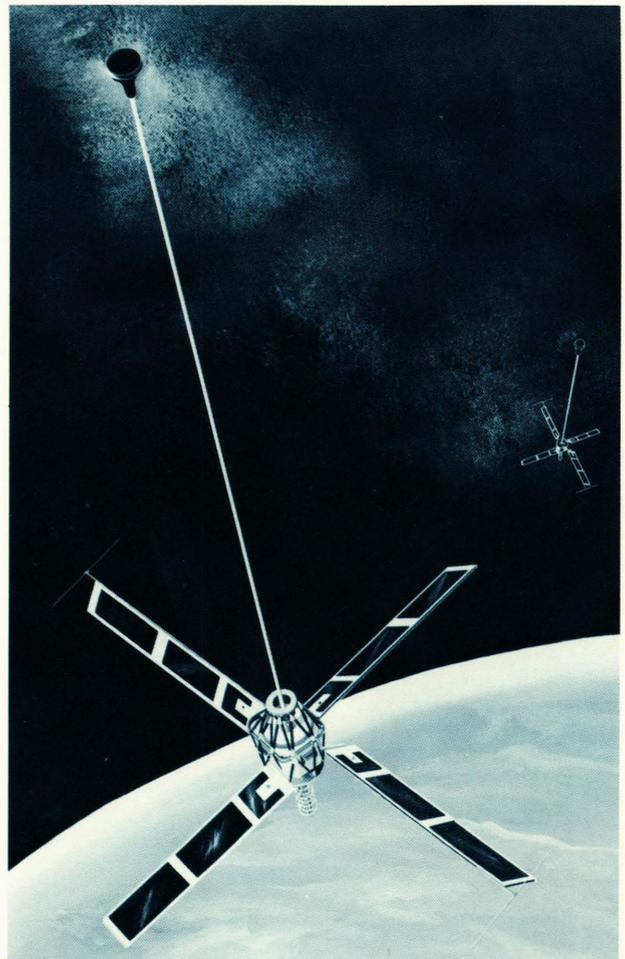
**Figure 6**—Orbit concept of the SOOS satellites. The lower OSCAR spacecraft (in the foreground) retains the graphite epoxy cradle that supports the upper OSCAR spacecraft (in the background) during the launch mode. The spacecraft are separated from the launch vehicle and from each other a short time after launch.
