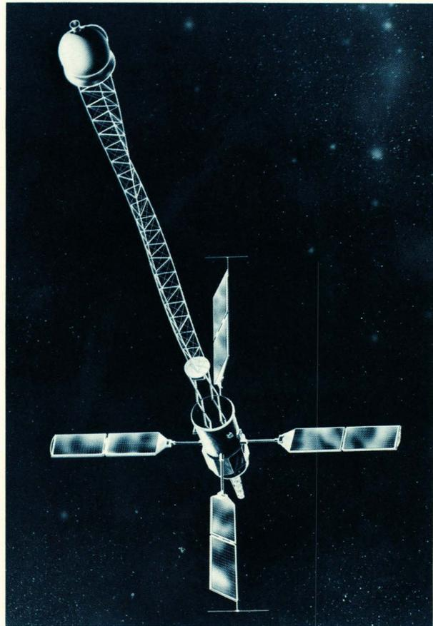
**Figure 4b**—In-orbit concept of a NOVA satellite. The launch weight is 370 pounds and the orbit is 600 nautical miles (nominal). The spacecraft has a DISCOS subsystem to compensate for the variable air drag and plane solar pressure forces acting on the spacecraft.
