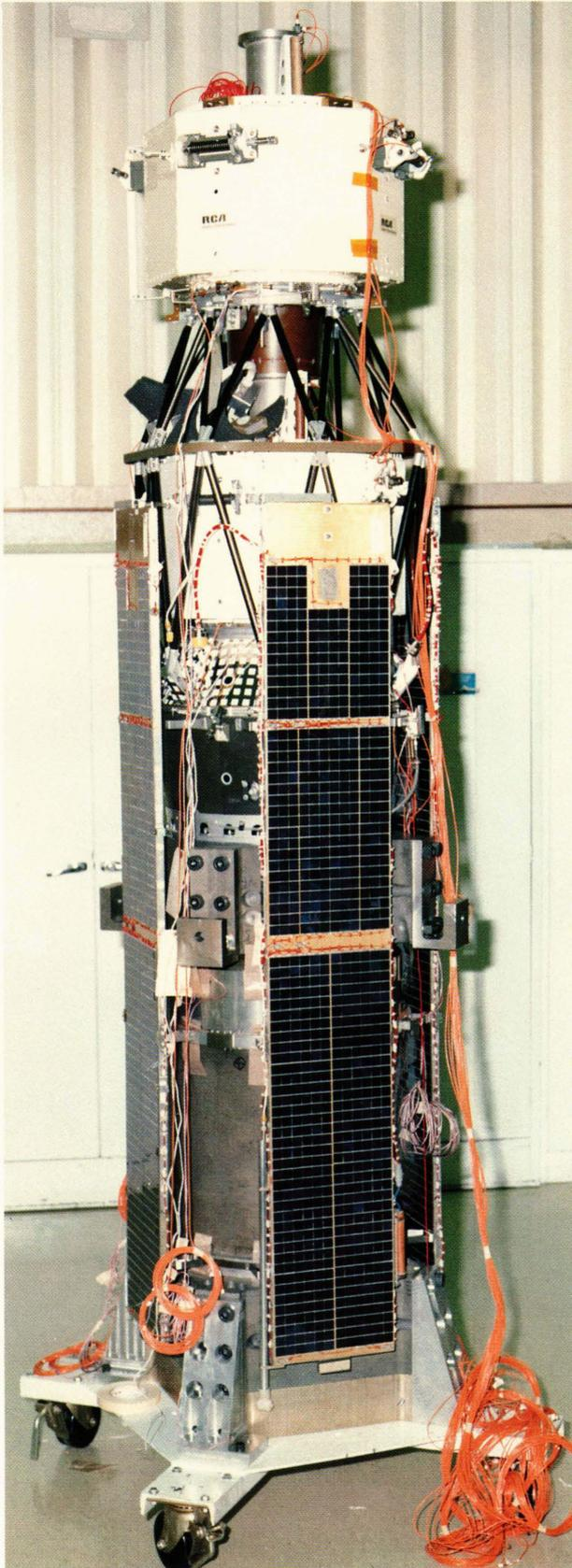
**Figure 7**—SOOS configuration on a simulated Scout rocket fourth stage. The upper spacecraft has the solar panels removed. (The wires are part of the test instrumentation.)
