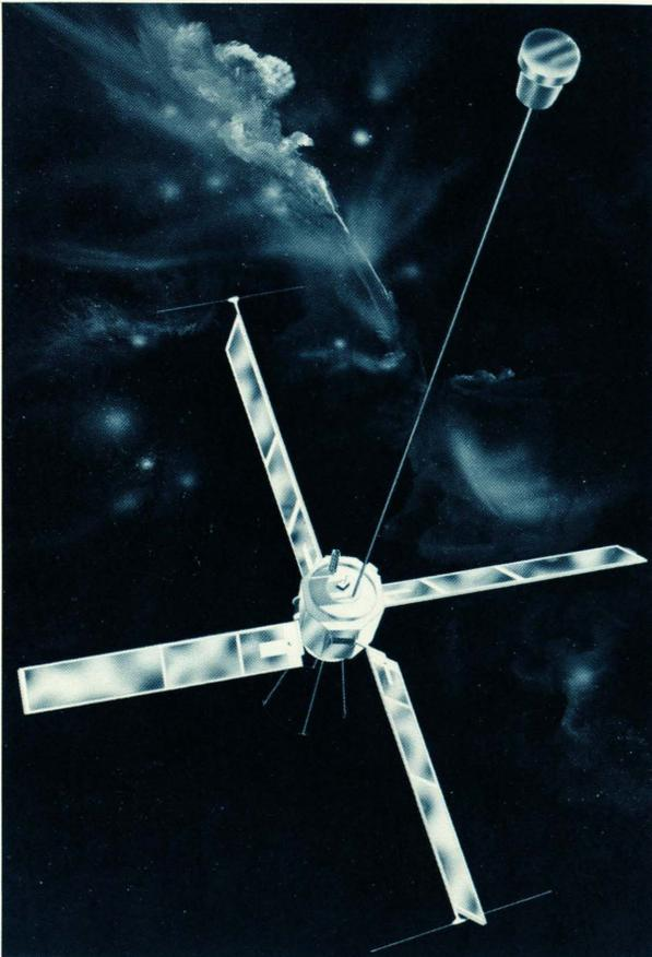
**Figure 4a**—Orbit concept of an OSCAR satellite. The launch weight is 130 pounds and the orbit is 600 nautical miles (nominal).
