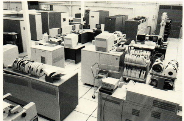
Figure 5—IBM 3033 multiprocessor, installed in 1979.
