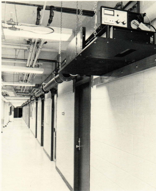
Figure 4 —The new apparatus under construction. The photon detection equipment and a vacuum chamber containing one end of the interferometer are in the foreground. The other end of the interferometer can be seen at a distance of 45 meters. The computer, control electronics, and an optical bench containing the light sources are located in a room at the far end of the hall.
