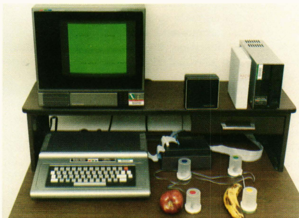
Figure 1 —This is the classroom MASH setup. I sat in front of the keyboard with the students, their switches, and attractors to my right. The switches connect to an input/output device, which is the larger black box behind the blue switch. This special APL-built interface provides robotic speech via a computer program, a synthesizer (mounted below the table to reduce television interference), and the small black speaker on the top shelf. The disk drive and its program-pack interface share the Color Computer's single programmable read-only memory port. The teacher can activate the switches from the keyboard, and either the student or teacher can make them light up and ring like a bell.
