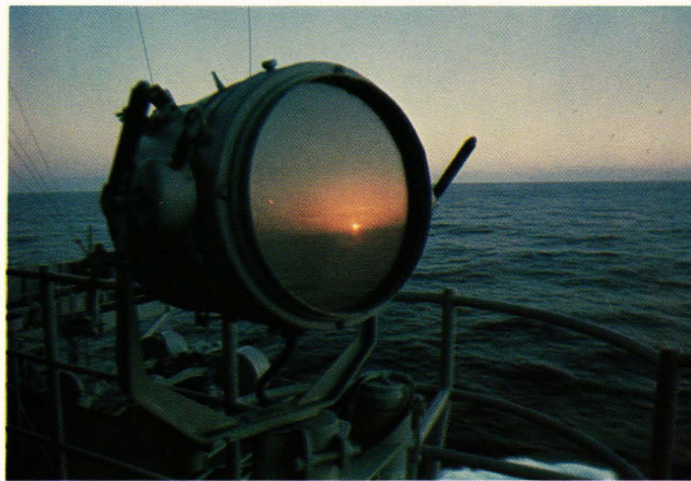
The venerable signal light continues to be an important element of the Navy C 3 system. During periods of emission control, it still provides a means of secure line-of-sight communications, free of jamming.
