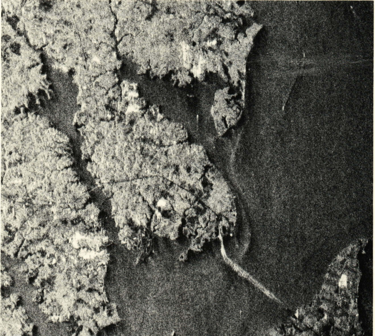
Figure 12a — Chesapeake Bay as observed on September 28, 1978, with the Seasat L-band SAR. The Naval Academy and the city of Annapolis can be distinguished southwest of the twin spans of the Bay Bridge that extends eastward to Kent Island. A tanker south of the Bay Bridge is evidently anchored there since no wake is apparent. Several smaller vessels in the upper portion of the scene do have wakes behind them, and the fastest moving of the group appears to be Doppler shifted off its wake. This scene was processed by the digital correlator at the Jet Propulsion Laboratory and was recorded on film in the APL Image Processing Laboratory using the Optronics P-1700 filmwriter to expose each of 10^7 picture elements.
