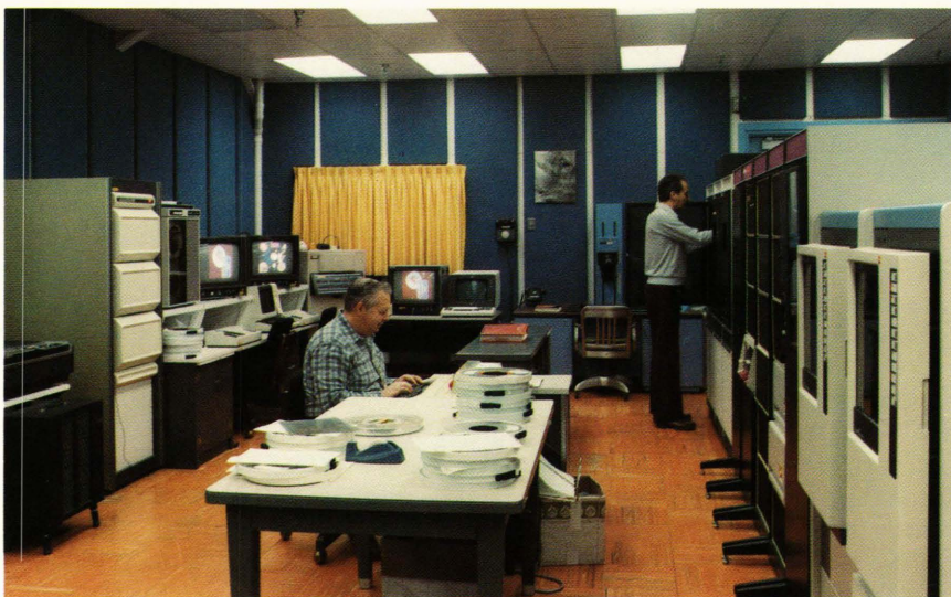
Figure 1 — A partial view of the APL Image Processing Laboratory showing the Comtal system (left foreground), Matrix camera (left rear), Grinnell workstation (center background), PDP-11/70 computer (right foreground), and Dicomed system (right rear).
