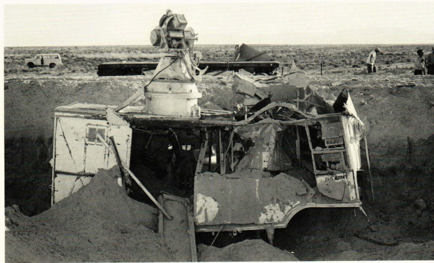
Figure 20 — A Talos ARM flight test conducted in October 1965 at White Sands Missile Range is illustrated by the sequence of pictures: (a) just before intercept of radar target, (b) impact and warhead detonation, (c) radar target after intercept. The damage mechanism is the warhead explosion plus the kinetic energy of the missile at impact.
