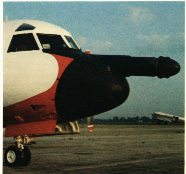
Figure 3 — Radiometer installation on RP-3A aircraft. The optics unit of the radiometer is mounted in a pod located above the radome of the aircraft. The forward extension and airstream control surfaces minimize air velocities within the pod.
