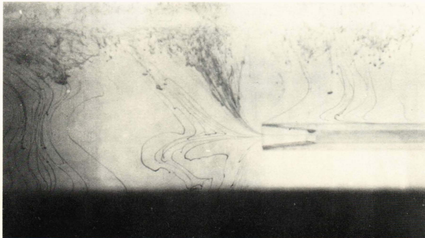
Figure 3 — Dye streak deformation patterns indicative of flow into the OTEC warm-water inlet. Dye streaks were initially vertical. Patterns indicate that the inlet will not capture water from the lower, colder layer, simulated by a dense, dark layer below the inlet.
