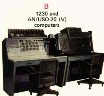
Figure 3 — CSEL Computer Center. The Computer Center contains the computers necessary to drive the tactical consoles in the Operations Center and to host computer program development. Specifically, the Center contains AN/UYSK-7, both single-bay and four-bay configurations, AN/UYSK-20, UNIVAC 1230, and AN/USQ-20 computers.
