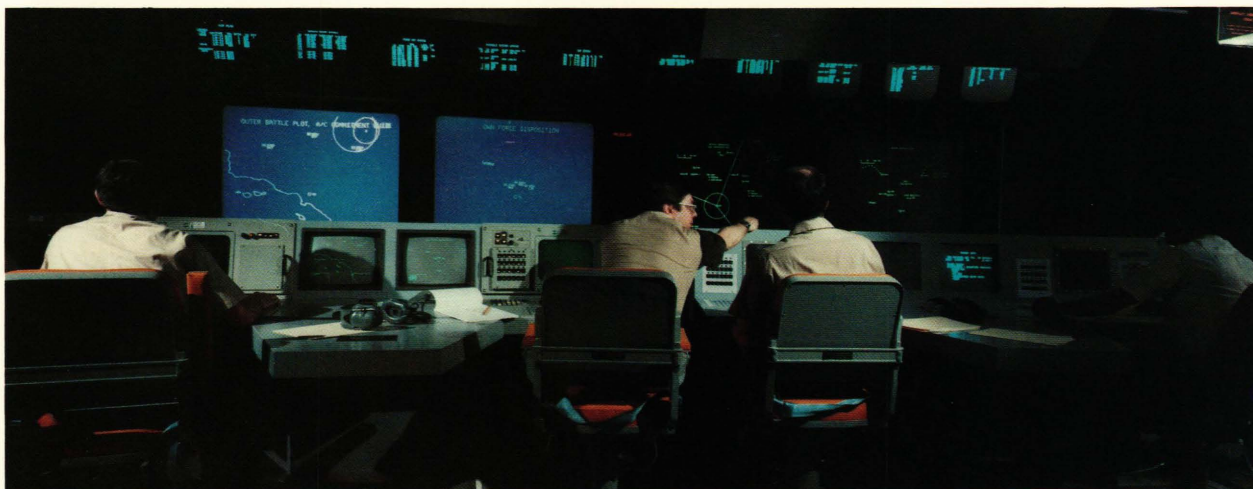
Figure 2 — Command display complex. The AEGIS Combat Information Center will include a command display complex. This center functions as an information management system designed to support ownship command and the Battle Group Anti-air Warfare Commander. It consists of four large-screen displays, ten alphanumeric displays, and four console-mounted high-resolution graphics monitors.
