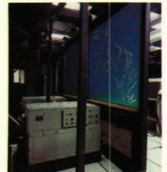
Figure 1 — CSEL Operations Center. The Operations Center contains much of the tactically significant equipment found in a shipboard Combat Information Center (CIC). It was used as an aid in determining the layout of AEGIS CIC's. The Operations Center is currently arranged as an AEGIS cruiser CIC.
