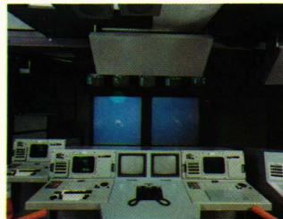
Figure 1 — CSEL Operations Center. The Operations Center contains much of the tactically significant equipment found in a shipboard Combat Information Center (CIC). It was used as an aid in determining the layout of AEGIS CIC's. The Operations Center is currently arranged as an AEGIS cruiser CIC.
