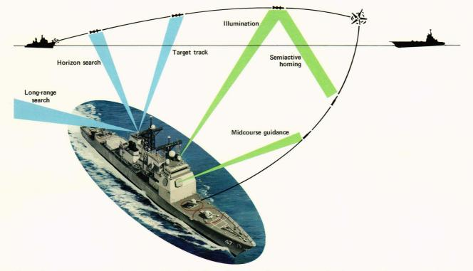
**Figure 4** — The AN/SPY-1A radar is a multifunction three-dimensional weapon control radar system that supports the engagement of air and surface targets from detection through interception. The operational sequence of events is illustrated here.
