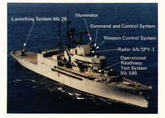
**Figure 6** — AEGIS Engineering Development Model 1 was installed in USS NORTON SOUND, where extensive tests and evaluations of the weapon system have been conducted since 1974.
