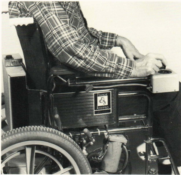
Fig. 1—Standard two-axis joystick for control of powered wheelchair.
