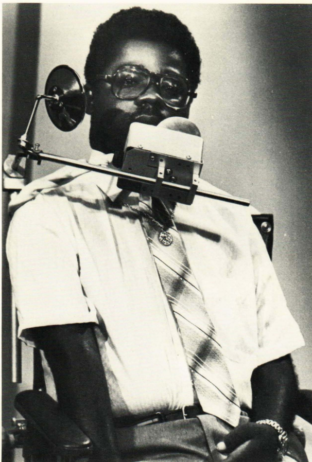
Fig. 2—VA chin controller for a powered wheelchair.
