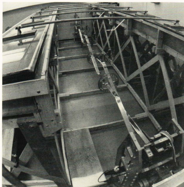
Fig. 2—The Magsat magnetometer boom float system. The magnetometer boom is suspended from floats in 6.1 m long flotation tanks that provided zero-g simulation in the horizontal plane. The boom was rotated about its longitudinal axis into four positions 90^\circ apart. Measurements of inclinations of sensor platform-mounted mirrors provided data that were used to align the mirrors by operating the gimbal at the base of the boom or by shimming the vector magnetometer base at the sensor platform end. Final measurements, adjustments, and checks were made by the attitude transfer system with the instrument module mounted on the rotary fixture.
