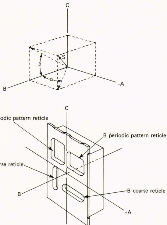
**Fig. 5—The precision sun sensor resolves the orientation of the sun line into two angles ( $\alpha$  and  $\beta$ ) in the sensor coordinate system by means of the A and B reticle assemblies. The periodic patterns determine the  $\alpha$  and  $\beta$  angles with a precision of 2 arc-s in a  $2.2^\circ$  repeating pattern. The coarse reticles determine which one of the  $2.2^\circ$  segments (in the  $32^\circ$  field of view) actually contains the sun line.**
