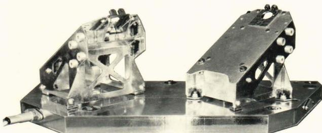
**Fig. 7—The Magsat optical bench shown here was fabricated by the Convair Division of General Dynamics. The inclined planes on the top surface hold the star cameras. The ADS components are mounted on the underneath side as illustrated in Fig. 1. The silver-like surface of the structure is the aluminum moisture barrier.**
