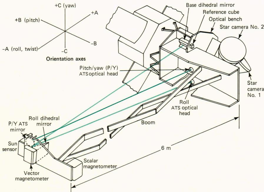
**Fig. 1—The attitude determination system consists of two star cameras mounted on an optical bench, which also contains an attitude transfer system for relating the orientation of the star cameras to the vector magnetometer. The sun sensor (and a rate gyro located in the spacecraft) provides additional information to allow interpolation between star sightings.**
