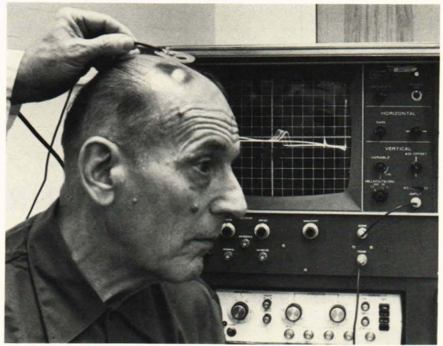
Fig. 3— Measurement of the ICP sensor in a patient with hydrocephalus. The pickup coil is held over the site of the implanted sensor. The display on the oscilloscope shows a pulse (one division to the right of the display's center) that indicates the RF absorption frequency of the sensor. The movement of this pulse is caused by ICP variations resulting from the heartbeat. The pulse at the 5th division is a 50 MHz calibration marker. The absorption frequency versus pressure of the sensor is known from previous calibration.
