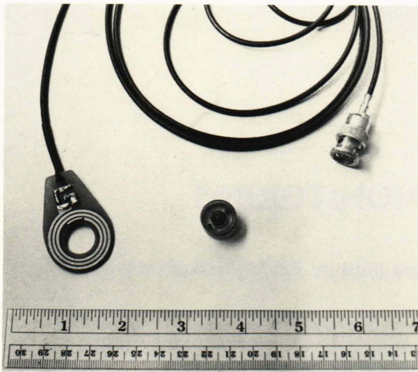
Fig. 2— The ICP sensor is shown in the middle of the photograph. The external pickup coil shown to the left of the sensor radiates a frequency modulated VHF radio signal. When the pickup coil is placed near the ICP sensor, RF energy is absorbed by the sensor at the resonant frequency of the tuned circuit inside the sensor.
