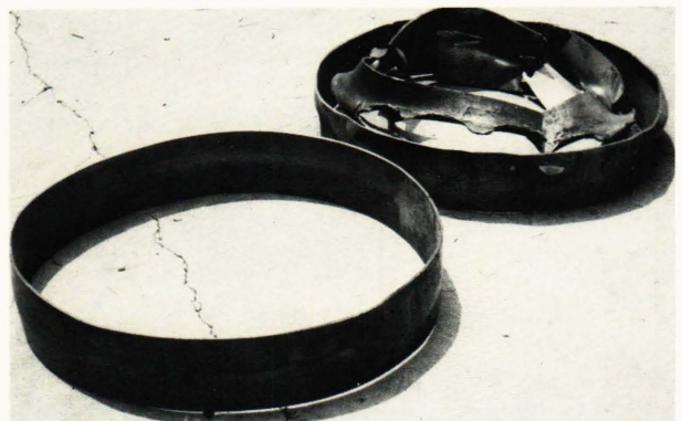
Fig. 2—Flywheel containment comparison between the APL-developed bare-filament configuration (foreground) and a typical laminated composite-disc flywheel (background).
