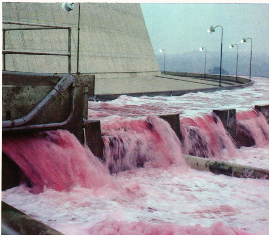
Fig. 6 —The cooling tower was charged to about 1 ppm with rhodamine (WT) dye, for the June 16, 1977 model validation test. Emissions from the cooling tower were traced.
