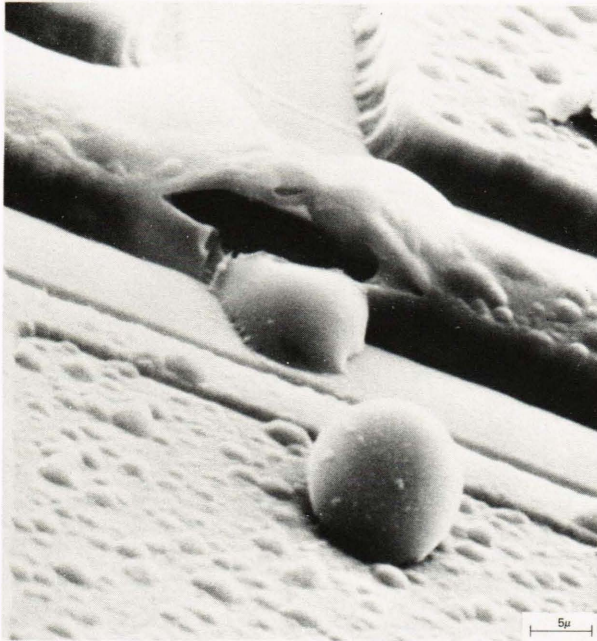
Fig. 2—An unusual failure of a hybrid circuit. The spherical piece of metal (aluminum, as shown by X-ray analysis) was spewed out of the crater that interrupts the metal track. An electrical failure was caused by the open track. The high spatial resolution and microanalysis capabilities of the SEM made this failure analysis possible.
