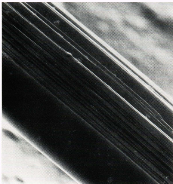
Fig. 9—SEM picture of HMTSF-TCNQ (magnification 2000). This is a top view showing evidence of macroscopic layering.
