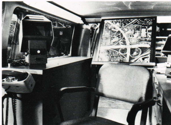
Fig. 23—Internal view of mobile command and control van with aerial photo board in position for use, with microfiche readers evident.
