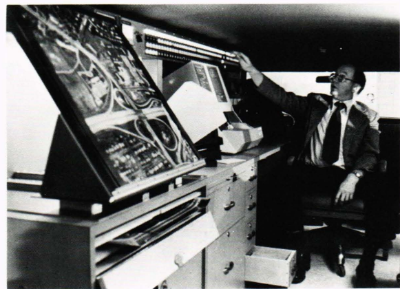
Fig. 22—Internal view of mobile command and control van showing aerial photo board and equipment status board, looking from back to front of the van.
