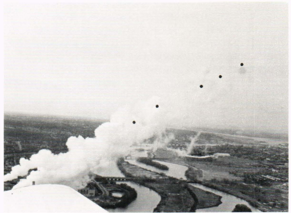
Fig. 7—Mechanical draft cooling tower plume at Benning Road as viewed from 305 meter altitude. The black dots indicate various altitude penetrations of the plume by aircraft.
