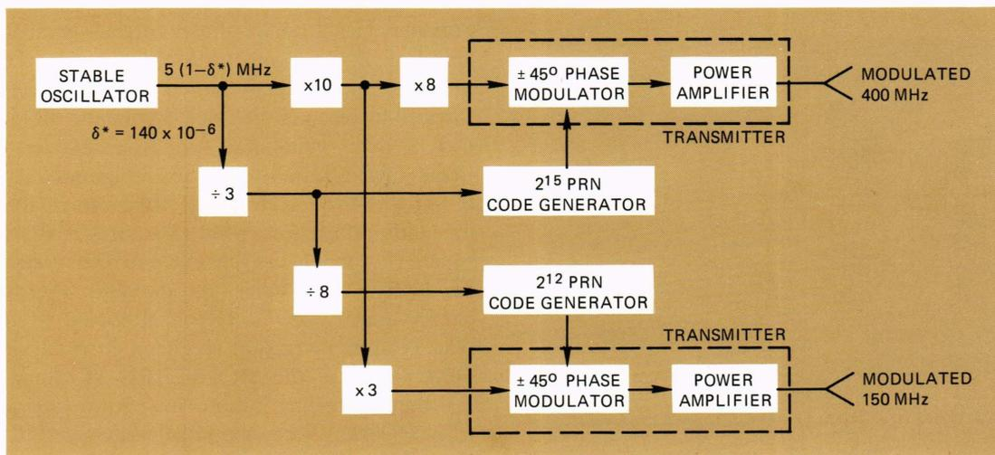
Fig. 1—TRIAD satellite RF system.
