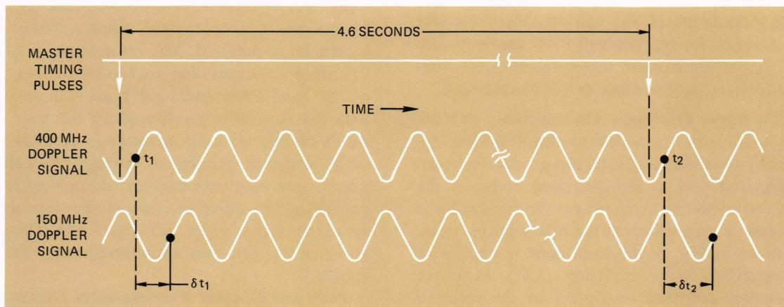
Fig. 6—Doppler measurement timing.
