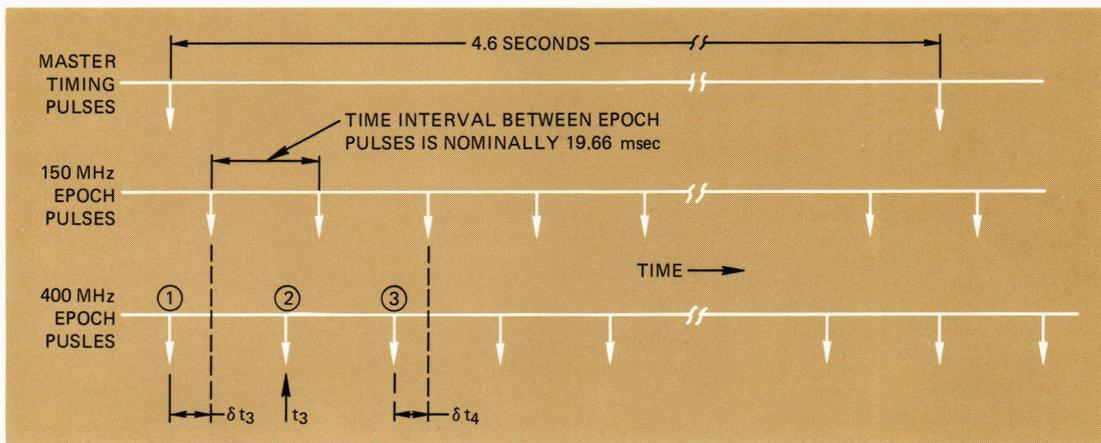
Fig. 7—PRN-ranging measurement timing.
