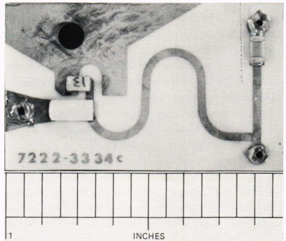
Fig. 3—TRIAD 400-MHz PRN phase modulator.
