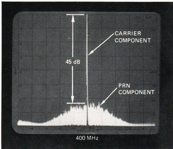
Fig. 4—Frequency spectrum of 400-MHz TRIAD transmission.
