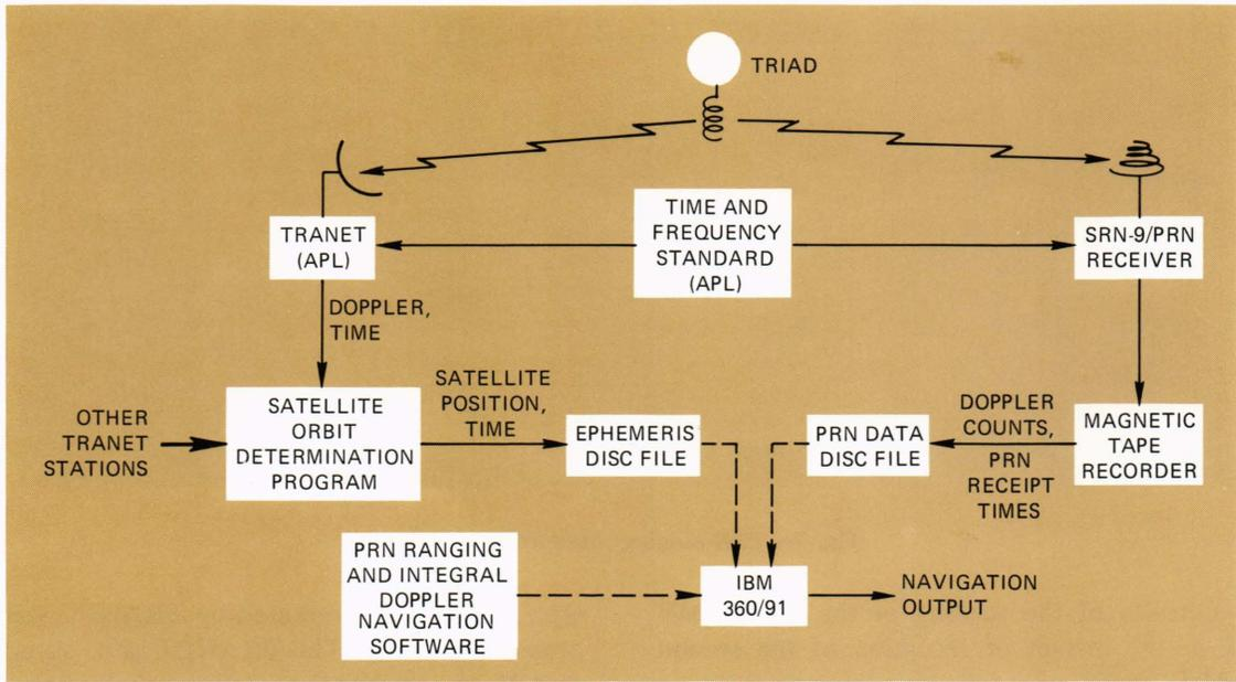
Fig. 8—Elements of the PRN data-gathering system.
