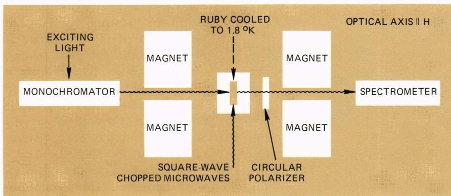
Fig. 3—Diagrammatic experimental setup for studying microwave-optical double resonance (MODR) at liquid helium temperatures. (The APL Microwave Physics Laboratory is equipped with such a setup.)
