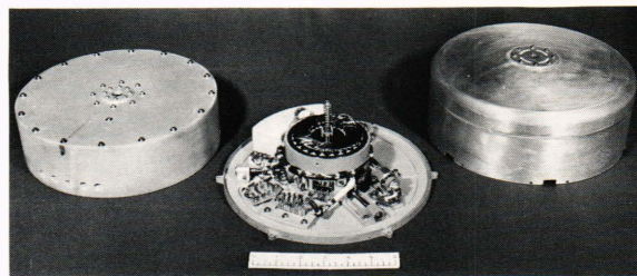
Fig. 1—Momentum wheel (disassembled); wheel, motor and caging mechanism, and cover.
