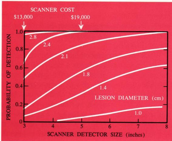
Fig. 6—Probability of detection of lesions as a function of scanner detector (crystal) size.
