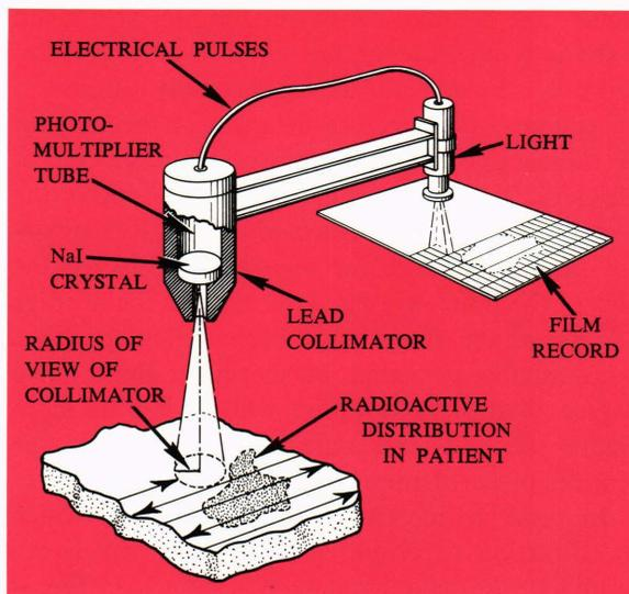
Fig. 4—Diagram of a typical rectilinear scanning instrument.
