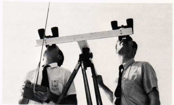
Fig. 6—Simple optical tracker mounted on camera tripod. Pilot is at left and tracker is at right holding handle.
