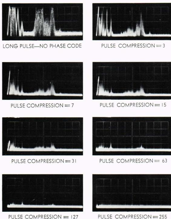
**Fig. 8—Detected video out of digital pulse compressor on rainstorm (100  $\mu$ sec/cm common to all).**
