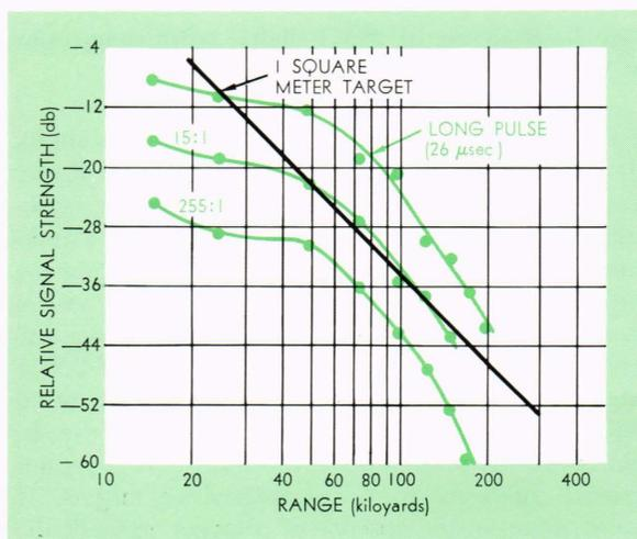
**Fig. 9—Snow clutter profiles for three compression ratios. Condition dry snow ( $\sim$  1 mm/hour water equivalent).**
