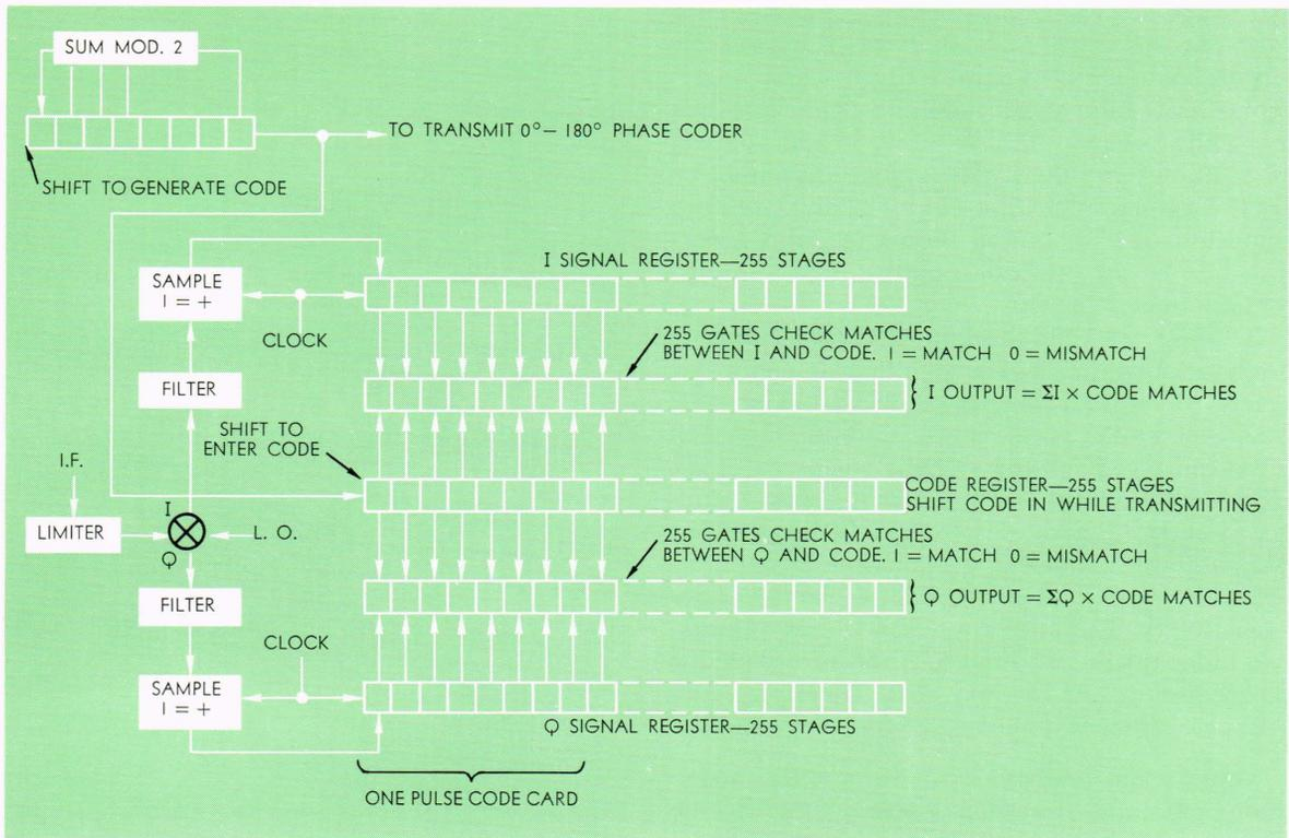
Fig. 2—Block diagram of digital compressor.
