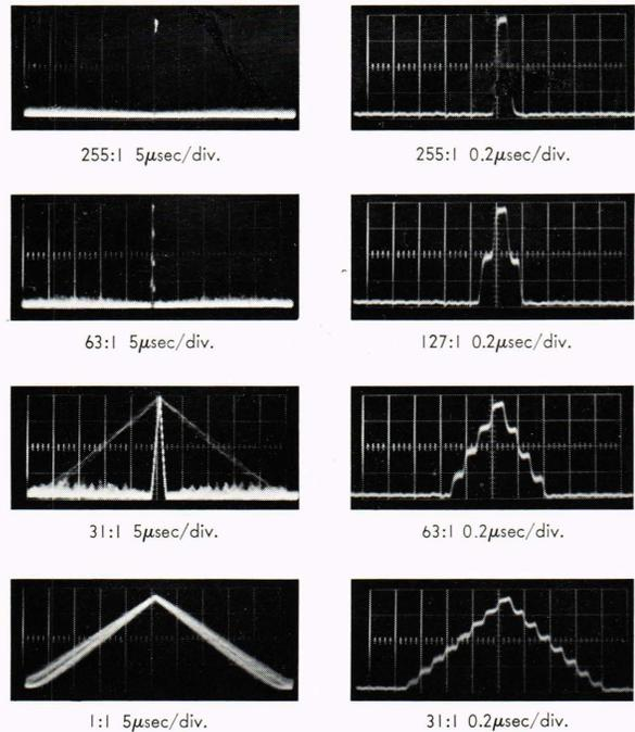
Fig. 4—Pulse compression outputs for varying amounts of pulse compression.
