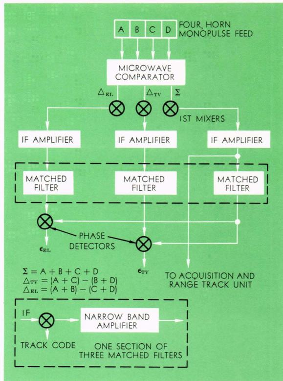
Fig. 5—Monopulse angle error processing system.
