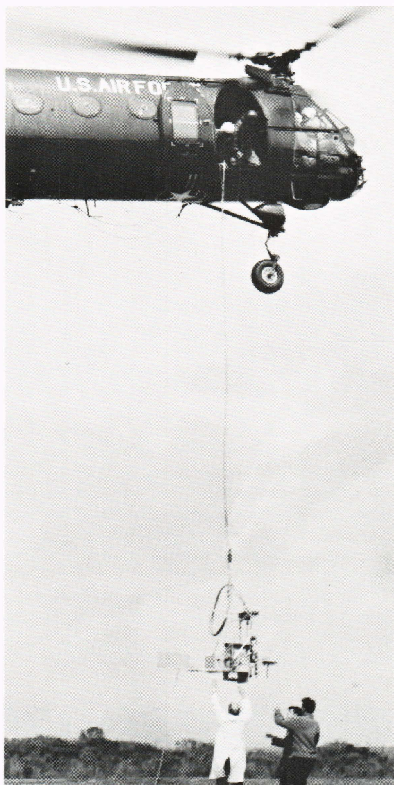
Fig. 5—Helicopter and refractometer package being launched. During measurements the package is suspended in undisturbed air about 85 feet below the helicopter.
